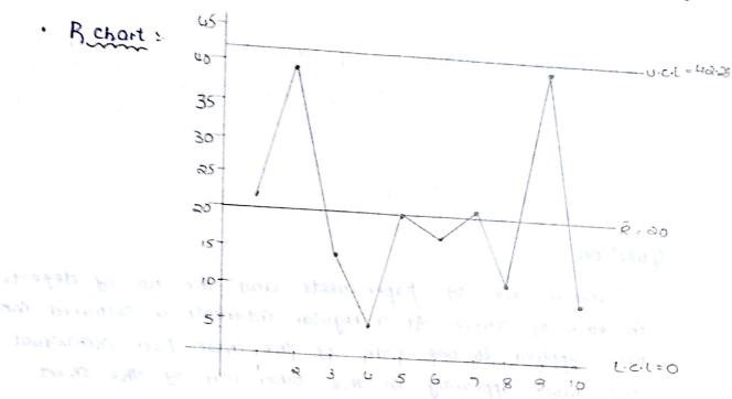
All the points are in between UCL and LCL so the process is in Control.
