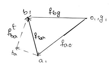
Acc. of B sel. to 0 = Acc. of B sel. to A + Acc. of A sel. to 0,  $f_{bo} = f_{ba} + f_{ao}$   $f_{bg} = f_{ao} + f_{ba}^{c} + f_{ba}^{t}$   $g_{bi} = o_{i}a_{i} + a_{i}b_{a} + b_{a}b_{i}$
