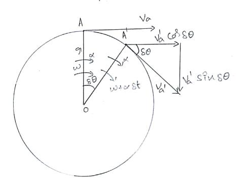
It has an angular velocity we and an angular acceleration of the same direction, the the angular velocity increases in the clockwise direction.
