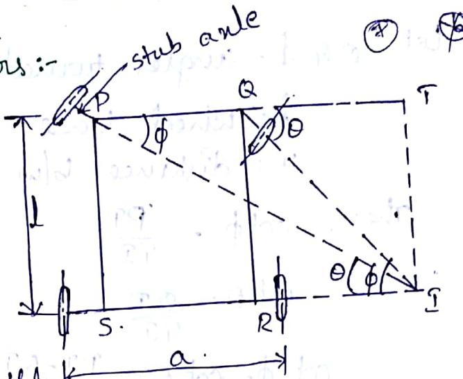
This is achieved by mounting the two front wheels on two short axles, known as stub axles. The stub axles are pin-jointed with the main front axle which is rigidly attached to the rear axle. Thus, the steering is affected by the use of front wheels only.
