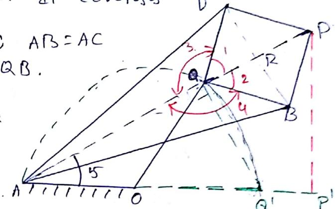
As link  $OQ$  rotates around  $O$ ,  $P$  moves in a straight line  $\perp$  to  $OA$ .
