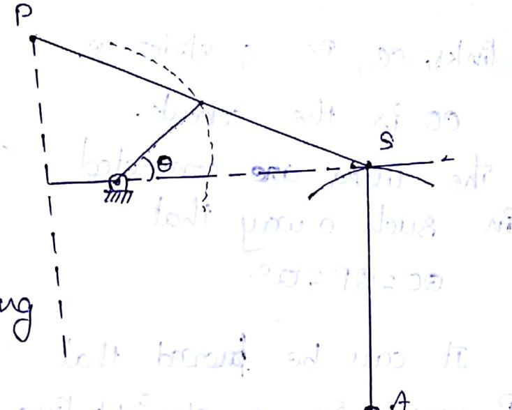
This is achieved by replacing the slider with a link AS in its mean position. AS is pin-jointed at A.
