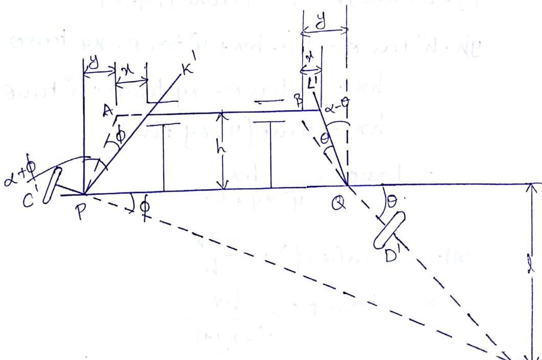
During the straight motion of the vehicle, the gear is in the mid position with equal inclination of the arms PK & QL with PQ.
