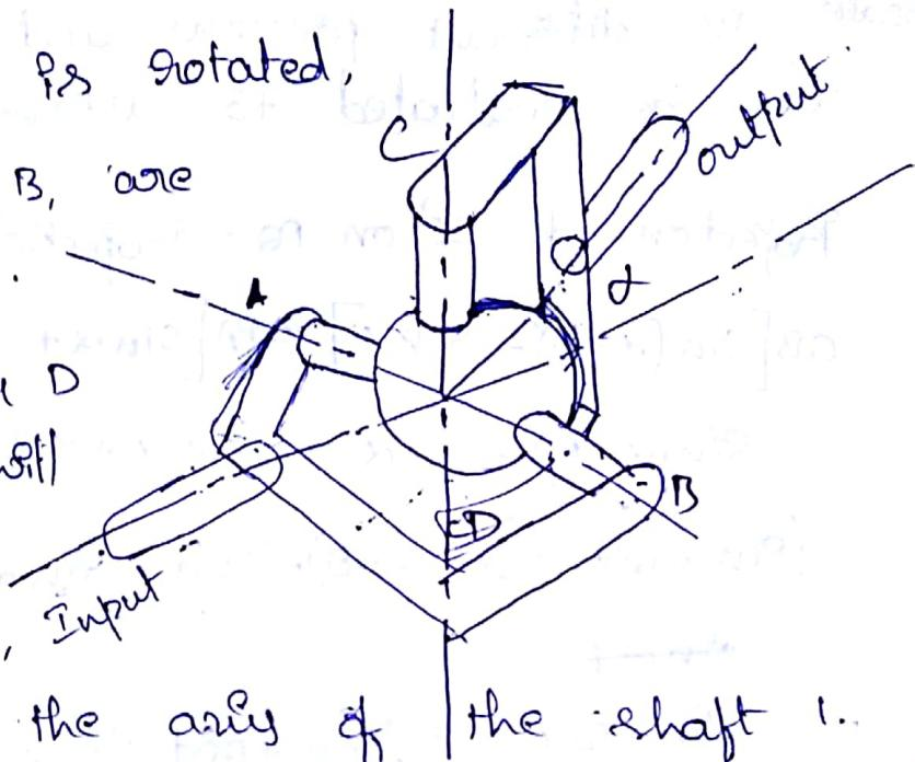
move in a circle. The point 'C' lies on a circle at the same height as it is on the ellipse. This gives the true angle of turned by the shaft 2.
