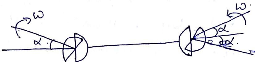
Two parallel & intersecting shafts may be connected by a double universal joint and have uniform output motions, provided that the intermediate shaft makes equal angles with the connected shafts and that the forks on the intermediate shaft are in the same plane.
