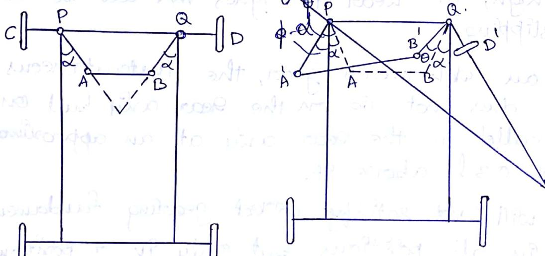
It is consisting of 4-link mechanism
