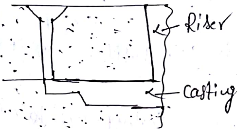
(a) Simple Parting line gate
