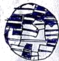
Structure of cartridge brass
