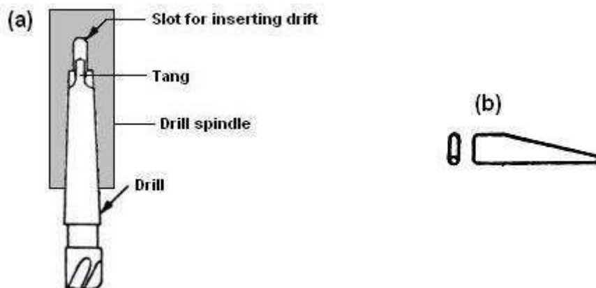
Fig. 3.122 (a) Drill directly fitted in the spindle and (b) Drift or key
