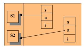
2. Assignment operator is used to assign the string to the variable s3. in this case, JVM first of all checks whether the same object is already available in the string constant pool or not. If it is available, then it creates another reference to it. If same object is not available, then it creates another object with the with the content "PREM" and stores it into the string constant pool.
