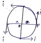
statement:- The line integral of Magnetie field intensity (ti) at any closed fath [solenoid, square, conducting wire or circular coil] is equal to the current enclosed by that Path.
