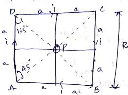
a steady direct current carried by loop it in requires to determine the magnetic-field intensity at point p at lentre of square.
