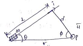
consider a straight wire of length l' carrying a steady current I. here we find the magnetic field intensity it at point p', with a distence of d' from the wire as shown in fig:
