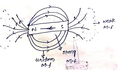
The region surrounding a Magnet in which the force by the magnet can be caperienced a field that is called a magnetic field it is indicated by ti. AmpTum/mt www.Jntufastupdates.com
