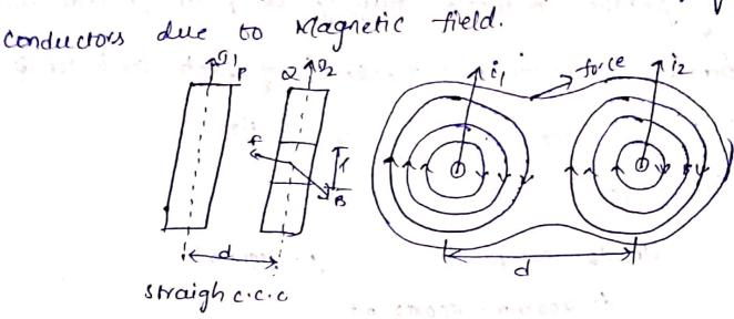
WKT Magnetic field intensity due straight cicic is, H = II [-for p-conductor]
