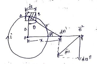
consider a circular loop of a radius a camping a cument ians we have to find the magnetic field intensity out fourt pon the oxis of loop with a distance of x nt. from its centre of consider a segment AB whose elemental lengths is 'de', let r be the distance of the element from points on 0 be
