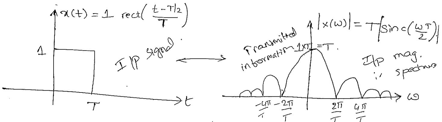
When we pass the <sup>rectangular</sup> IIP signal through a low pass filter, low pass filter allows only low frequency components of IIP signal and ~~not~~ attenuates high frequency components of IIP signal.
