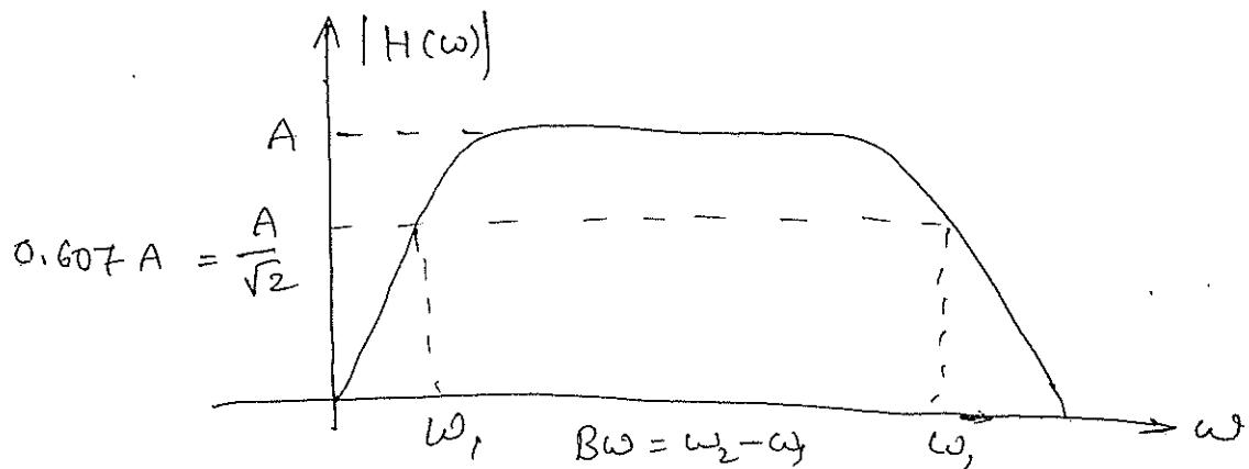
i.e) Bandwidth =  $(\omega_2 - \omega_1)$  as shown in fig.
