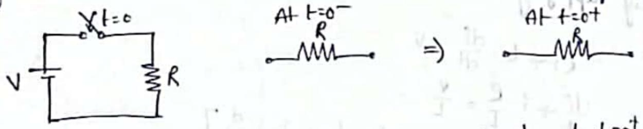
The governing equations of the network at  $t=0^+$  are obtained by using either KCL or KVL with the help of these equations,  $\frac{di}{dt}$  and  $\frac{dv}{dt}$  can be evaluated.
