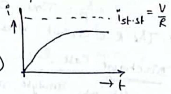
Note! Once the transient dies out within the short spell of time the steady state (st-st) current remains in the circuit is  $\frac{V}{R}$ .
