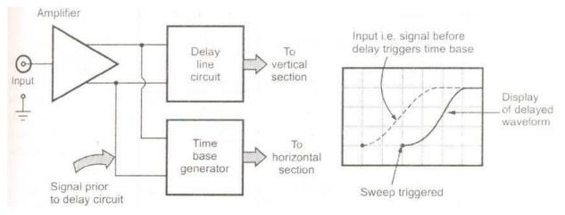
Due to triggering of time base by input signal, sweep starts well in time and when input appears at vertical sections, the sweep is triggered and delayed  $W(l \setminus dorm$  is displayed. The delay ensures that no part of the waveform gets lost.
