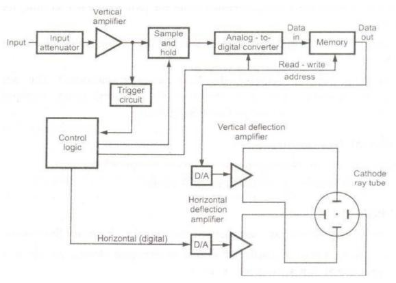
As done in all the oscilloscopes, the input signal is applied to the amplifier and attenuator section. The oscilloscope uses same type of amplifier and attenuator circuitry as used in the conventional oscilloscopes. The attenuated signal is then applied to the vertical amplifier.
