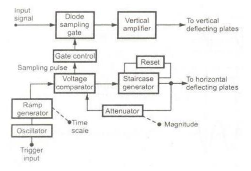
The input signal is applied to the diode sampling gate. At the start of each sampling cycle a trigger input pulse is generated which activates the blocking oscillator. The oscillator output is given to the ramp generator which generates the linear ramp signal. Since the sampling must be synchronized with the input signal freq, lency, the signal is delayed in the vertical amplifier.
