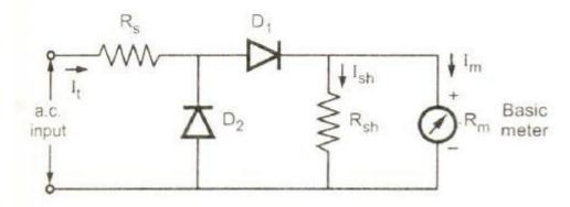
The diodes D1 and D2 are used for the rectifier circuit. The diodes show the nonlinear behaviour for the low currents hence to increase the current through diode D1, the meter is shunted with a resistance Rsh' This ensures high current through diode and its linear behaviour.
