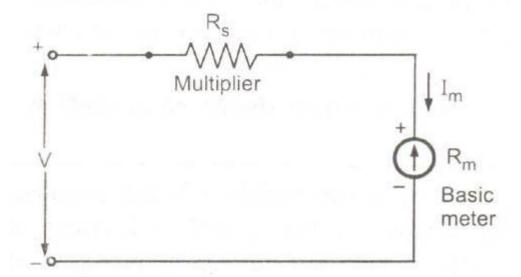
The voltmeter must be connected across the two points or a component, to measure the potential
