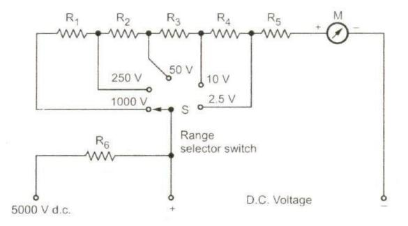
For getting different ranges of voltages, different series resistances are connected in series which can be put in the circuit with the range selector switch. We can get different ranges to measure the d.c. voltages by selecting the proper resistance in series with the basic meter.
