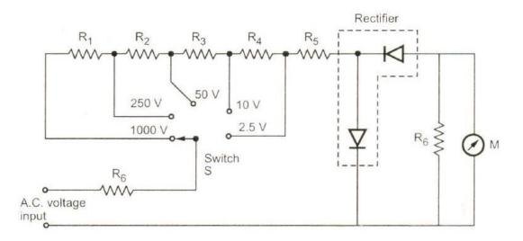
The rectifier used in the circuit rectifies a.c. voltage into d.c. voltage for measurement of a.c. voltage before current passes through the meter. The other diode is used for the protection purpose. Use of multimeter for resistance measurement:
