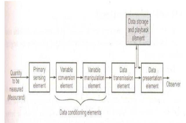
diagram instrument can be studied interms of these functional elements. The Fig. 1.1 shows the block
