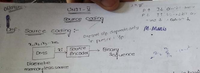
\* A conversion of discrete memory less source which is having Symbols 2, 122, ... 2m with the probabilities P(21), P(22), P(23)... ... P(xm) is converted in to a binasty code word (or) a bit sequence is called as source coding. \* The device which performs the conversion is called as source Encoder.
