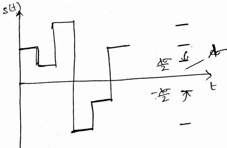
Fig:- A sequence of messages is represented by waveform  $s(t)$  which assumes voltage levels corresponding to the messages.
