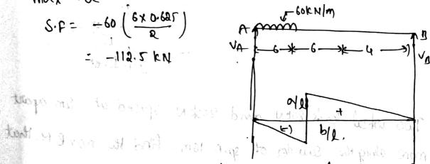
5. Two wheel loads 80 km and 200 km spaced 2m apout move on a swardday of span 16m find the max the s.p. and we sprata section un from the left end.
