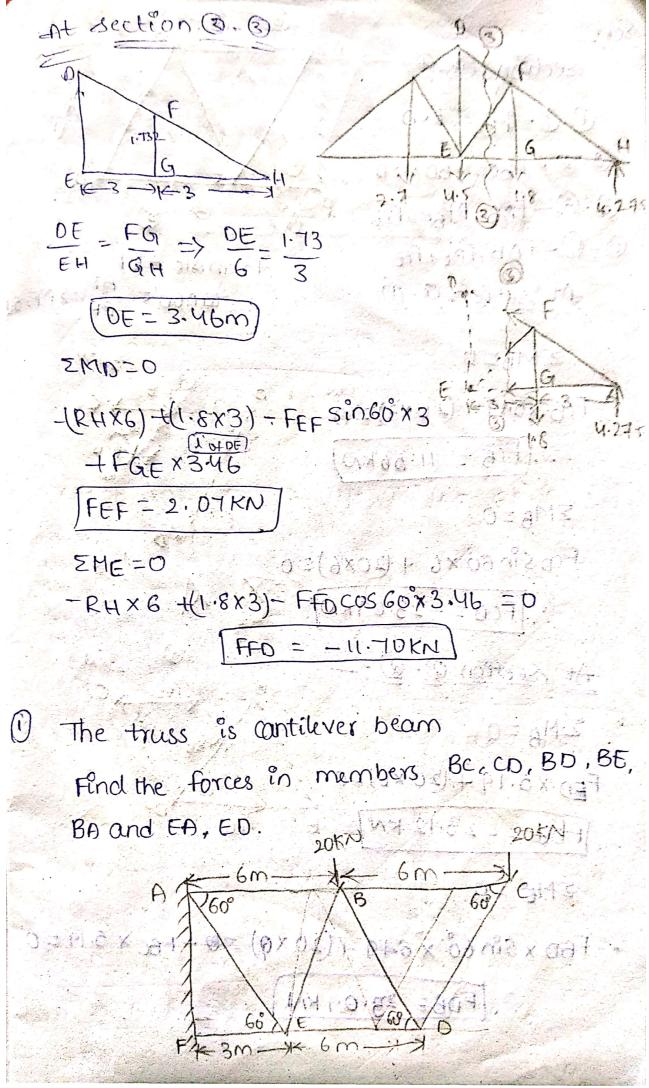
section O-O 1.0- FBC, FCD (J-D-FBC, FBD, FED 3-3- FAB, AFBE, FOE Q-Q-FAB, FAE, FFE tromale AEF -lango = AF => AF=5 h At setion Q-O ZMD=0 FCB x5.19+(20x3)=0 : (FCB = 11.56KN) EMB=0 Fasin 60 x6 + (20x6)=0 : FCO = -23.09 KN 1 / CVA At section Q-Q: - = cail ZMB =0 (mid savality) (FB0 31) FED X 5.19 + (20 ×6) =011/11/20160) JFOE = - 23.12 KN E / FLOS (1) 100 00 IME =0 - FBD x Sin 60 x 5.49 + (20 x 9) = - FBC x 5.19 = 0
