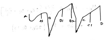
A continous beam ABC covers timo consequire spons AB and Be of length 4m and 6m carrying UDL of GKN/m and LOKN/m respectively it the ends A and c are simply supported find the support moments at A.B and c and draw B.m [0+90+30] [08-08 : giogram
