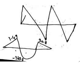
Determine the support moments at A, B, c and D for the gerden AB of Span 3m coorying a point load of 8kN at 1m distance from the left and Bc of Span 4m Coorying a UDC of 5kN-m through out the Bc Span. CD with the spain and 4m Coorying a point load 4kN at the center and the CD Span. A and B one fixed.
