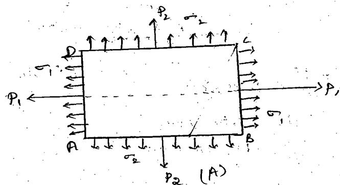
Let us consider a beam ABCD of uniform cross area 'A' with unit thickness subjected to 2 direct stresses as shown in fig (A).
