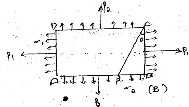
→ on section CF, the tensile forces are also acting where  $P_1$  is acting in axial direction and  $P_2$  is acting in downward direction.
