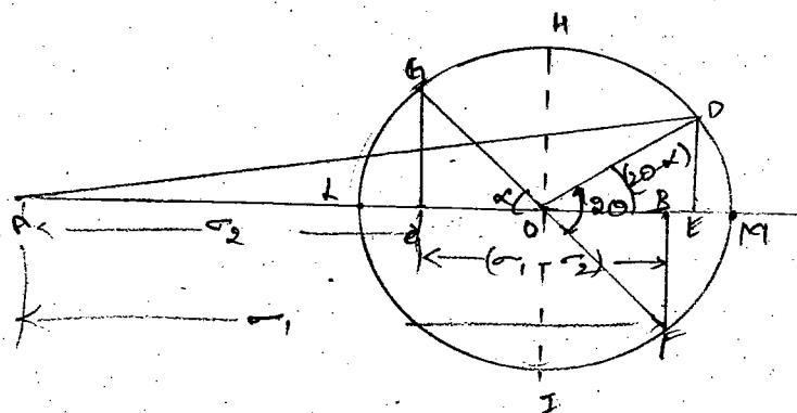
→ Let AB be any line which is representing major tensile stress draw right side of point and AC be any line drawn towards point A so that AC is minor tensile stress.
