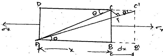
Strain in x direction on AB plane due to  $\sigma_x$  is given by,  $e_x = \frac{\text{change in length}}{\text{original length}}$
