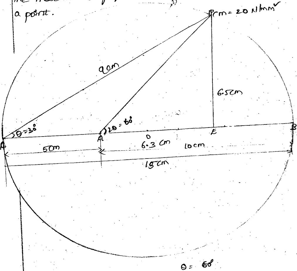
2. The stresses at a point in a part are 100 MPa and 75 N/mm<sup>2</sup> compression. Determine the normal stress, tangential stress, resultant stresses and obliquity on an inclined plane which is making an angle 38° with the mindal axis.
