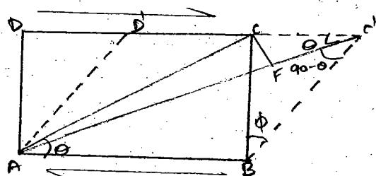
4. Strain on an oblique plane when body is subjected to stress in x-direction, stress in y-direction and these stresses are accompanied by shear stress
