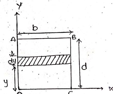
Consider a rectangular elementary strip of thickness "dy" at a distance "y" from the axis "Ox".
