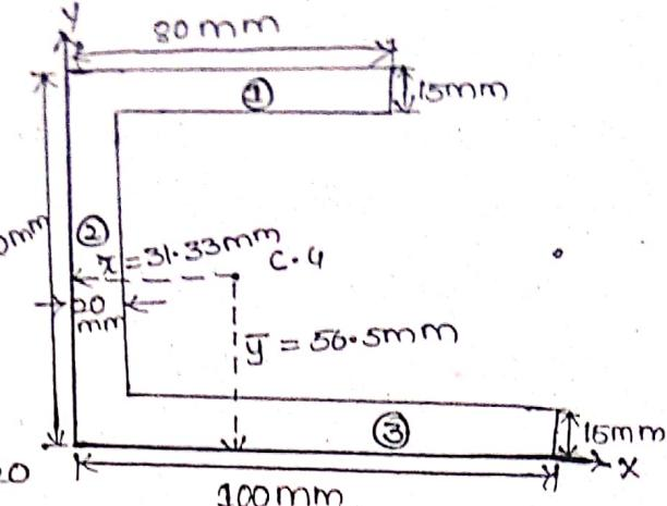
7. Determine the centre of gravity of the shaded area as shown in fig.
