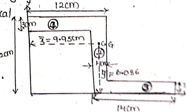
$$\begin{aligned} \text{Total area } A &= A_1 + A_2 + A_3 \\ &= 36 + 28 + 28 \\ &= 92 \text{ cm}^2 \end{aligned}$$
