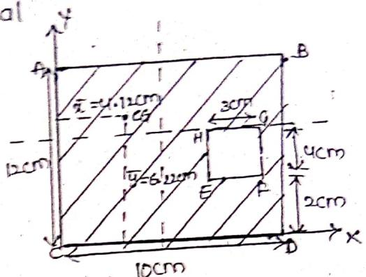
9. Find Centre of gravity of the composition figure given below.
